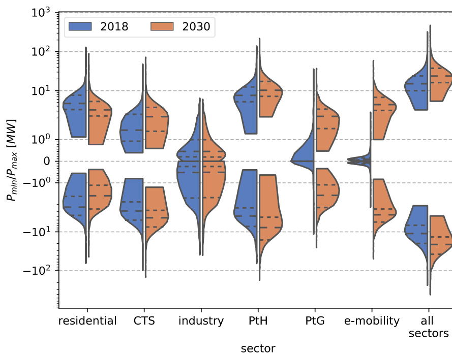
Figure 25 Distribution of the potential values for load increase, P_{max} (positive values), and load decrease, P_{min} (negative values) (Heitkoetter et al., 2021, p. 10).
